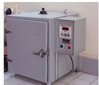
Figure 1.6. A Bacteriological incubator
